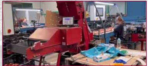
Since Fusarium can be detrimental to Tulip bulbs, especially after washing, new machines were invented to detect diseased bulbs by imagery so they can be eliminated early on. (One rotten apple can ruin the entire basket.)
