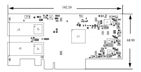
Mechanical Drawing of Dual-port 10/25 Gb/s Adapter Card
