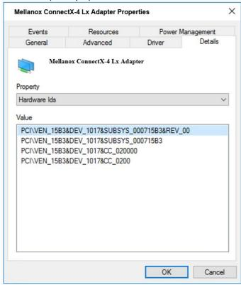
5. In the Value display box, check the fields VEN and DEV (fields are separated by '&'). In the display example above, notice the sub-string "PCI\VEN\_15B3&DEV\_1003": VEN is equal to 0x15B3 – this is the Vendor ID of Mellanox Technologies; and DEV is equal to 1018 (for ConnectX-4 Lx) – this is a valid Mellanox Technologies PCI Device ID.
