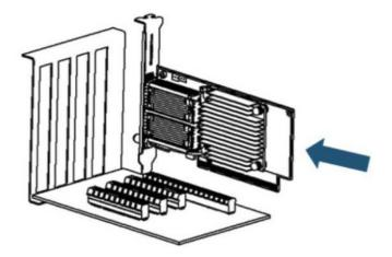
4. Applying even pressure at both corners of the card, insert the adapter card into the PCI Express slot until firmly seated.
