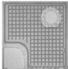
Conventional LED device with patterned sapphire substrate (PSS) (essentially all LED chip makers)
