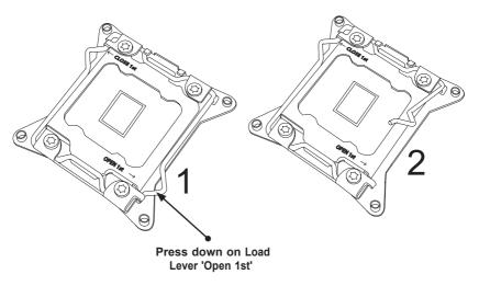
2. Press the second load lever labeled 'Close 1st' to release the load plate which covers the CPU socket from its locking position.
