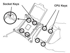
Use your thumb and index finger to hold the CPU on its edges. Align the CPU keys (semi-circle cutouts) against the socket keys.
