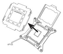
1. With the LGA 2011 socket open, remove the 'WARNING' plastic cap using your fingers.
