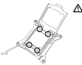
Warning: You can only install the CPU inside the socket in one direction. Make sure that it is properly inserted into the CPU socket before closing the load plate. If it doesn't close properly, do not force it as it may damage your CPU. Instead, open the load plate again and double-check that the CPU is aligned properly.
