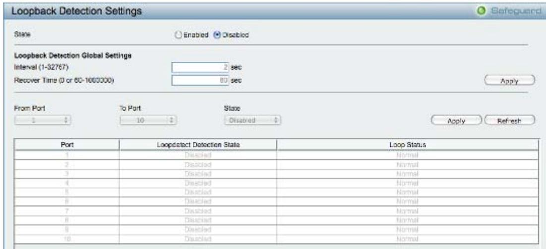
Figure 66 – Configuration > Loopback Detection
