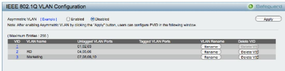
Figure 50 – Configuration > 802.1Q VLAN > Example VLANs
