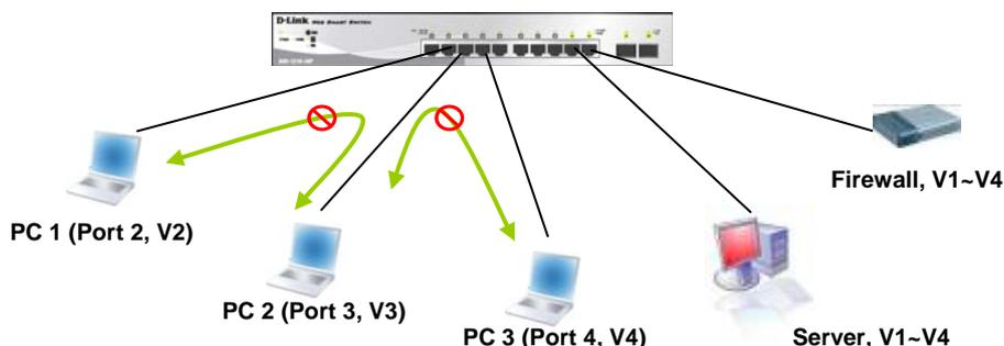
Figure 52 – Configuration > 802.1Q VLAN > Asymmetric VLAN Example
