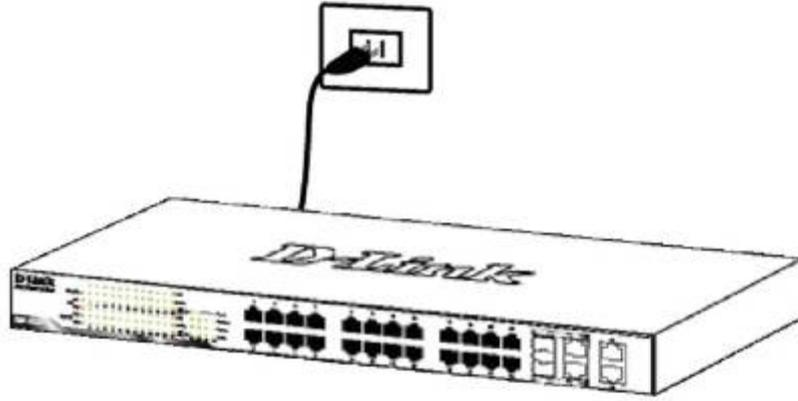
Figure 6 –Plugging the switch into an outlet
