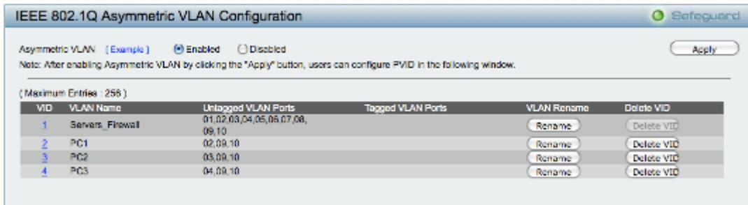
Figure 54 – Configuration > 802.1Q VLAN > Asymmetric VLAN – Create VLANs
