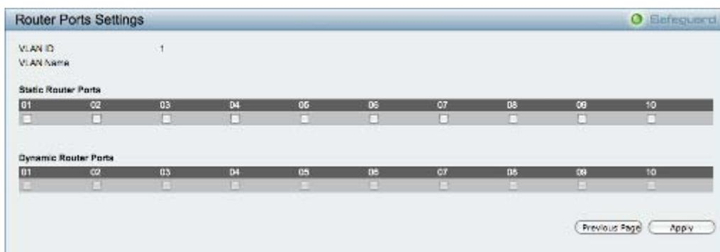
Figure 62 – Configuration &gt; IGMP Snooping &gt; IGMP Router port Settings
