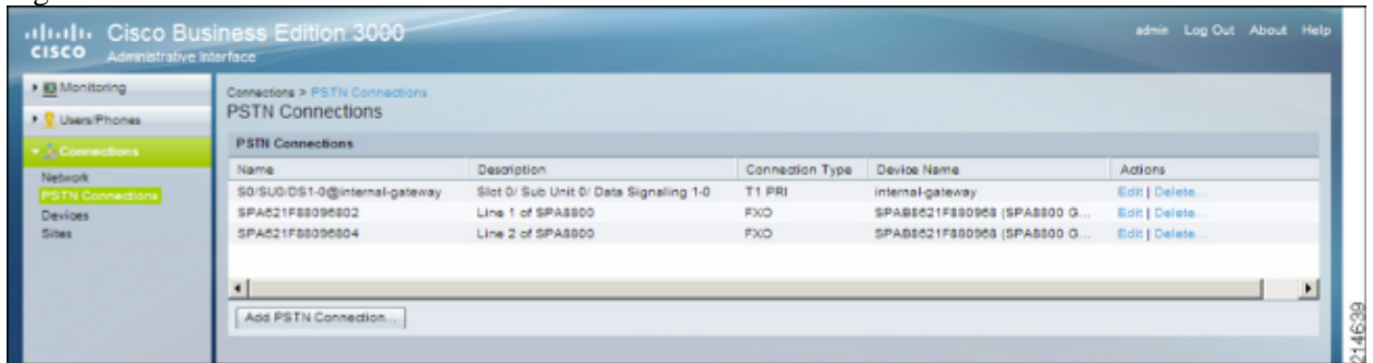
Figure 6 – FXO PSTN Connections on SPA8800 Listed in the Cisco BE3000
