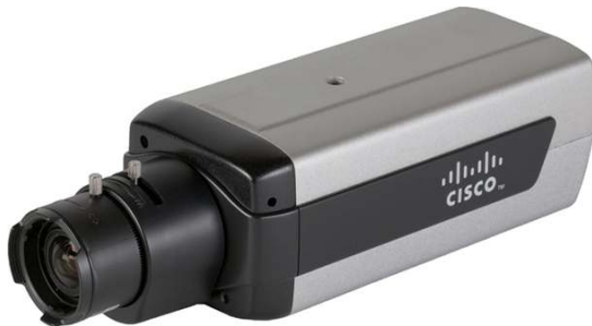
Figure 1. Cisco Video Surveillance 6000P IP Camera
