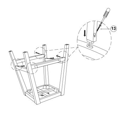
DO NOT FULLY TIGHTEN SCREWS (13)
