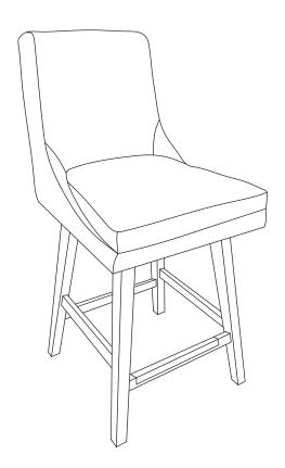
CAREFULLY TURN TO THE UPRIGHT POSITION. APPLY FIRM PRESSURE TO ALIGN. FULLY TIGHTEN ALL BOLTS (10) & SCREWS (13).
