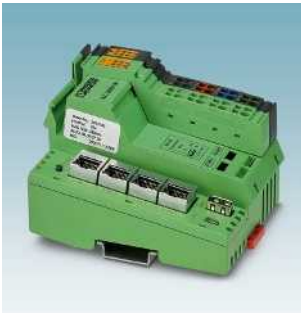
Controller for building infrastructure Page 79
