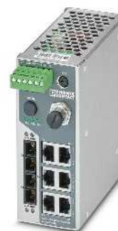
6 RJ45 ports and 2 fiber optic ports (single-mode)
