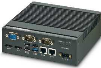
Box PC with Intel® Celeron® N2930 technology
