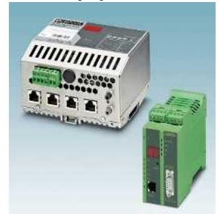
Proxies as a link between PROFINET networks and other fieldbus systems Page 444
