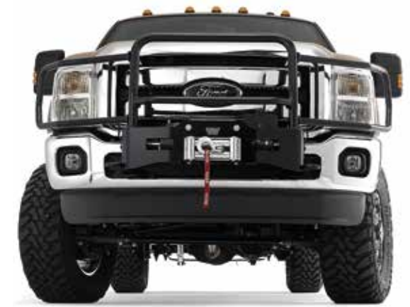
2011-15 Ford Super Duty equipped with WARN Gen II Trans4mer Mounting Kit, Grille Guard Tube (tall version), Headlamp Guards, and Light Bar
