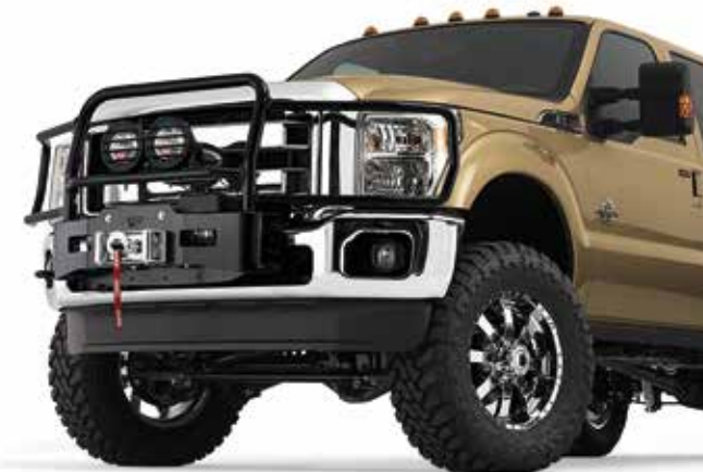
2011-15 Ford Super Duty equipped with WARN Gen II Trans4mer Mounting Kit, Grille Guard Tube (tall version), Headlamp Guards, and Light Bar
