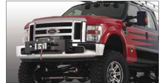
Gen II Trans4mer mounting kit, brackets, and 16.5ti winch
