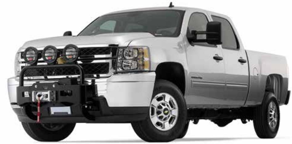
2011-13 Chevy Silverado 2500 equipped with WARN Gen II Trans4mer Mounting Kit and Grille Guard Tube (short version)
