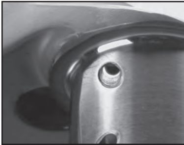
Looking from the rod, back up through the main, you can see daylight, indicating it's a genuine Crower crankshaft with the "straight-shot" oiling system.
