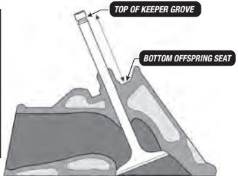
Diagram 1. Calculating Installed Spring Height
