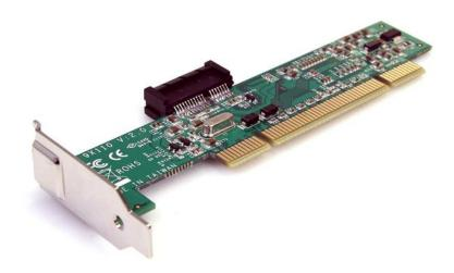
The PCI1PEX1 PCI to PCI Express Adapter card lets you use low profile PCIe expansion cards in a server/desktop motherboard PCI slot. The adapter connects through a 32-bit PCI slot to provide a low profile PCIe x1 slot in its place; a spare, full size bracket is included for installation in larger desktop or server expansion slots that can accommodate a full-sized card.
