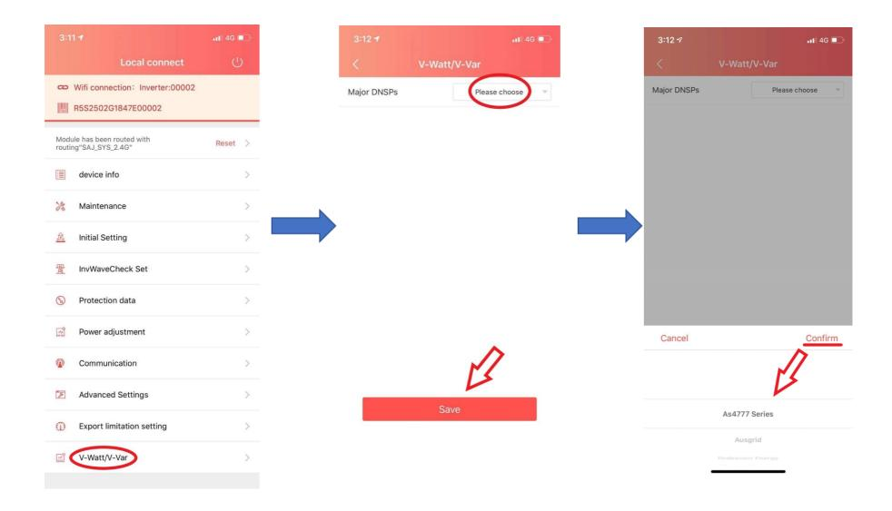
Step 4-2: Then tap 'Save' at the bottom of the page. After a few seconds, it will show a dialog box to remind to restart the inverter, then tap 'RESTART NOW' .The inverter will restart, and V-Watt/V-Var setting is completed.
