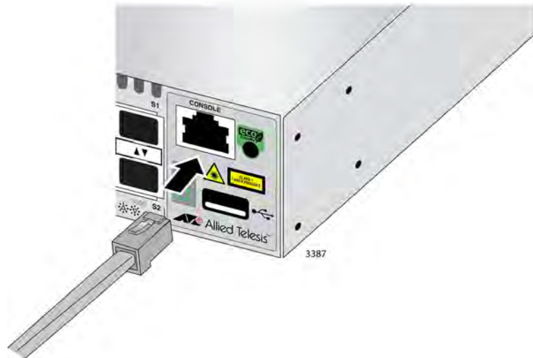
Figure 33. Connecting the Management Cable to the Console Port
