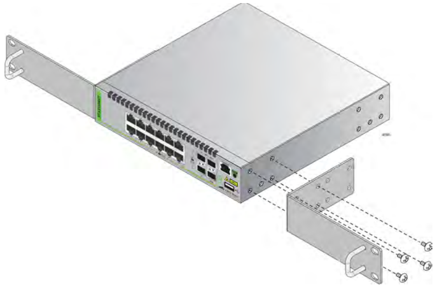
Figure 14. Installing the Brackets on the Switch
