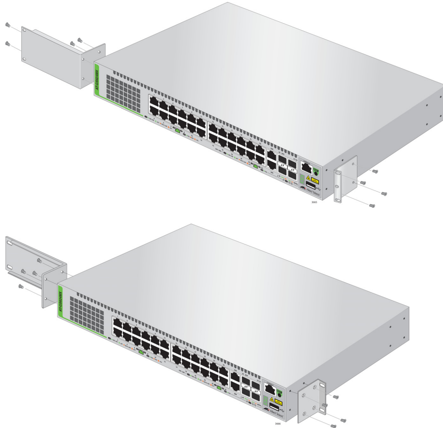
Figure 25. Installing Brackets on the AT-GS924MX Switch
