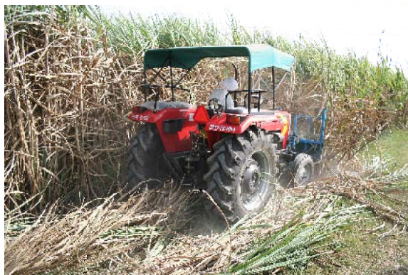
Fig. 7.2: Tractor operated front mounted sugarcane harvester in operation
