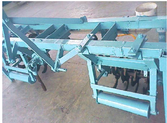
Fig.7.5: Residue mulcher-cum-bio applicator
