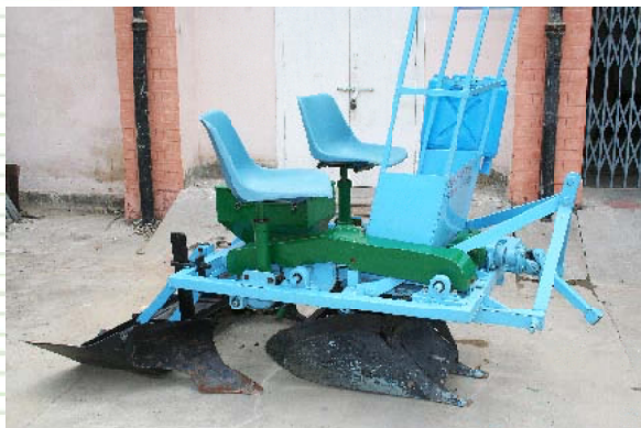
Fig. 7.4: Side view of paired row sugarcane cutter planter with attachments for furrow making at both ends of paired row
