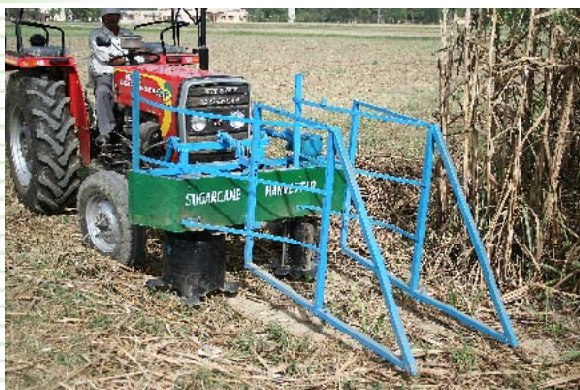
Fig. 7.1: Tractor operated front mounted sugarcane harvester
