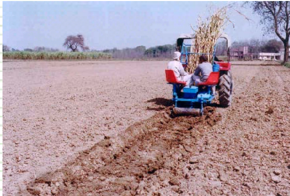
Fig. 7.3: Paired row sugarcane cutter planter in operation
