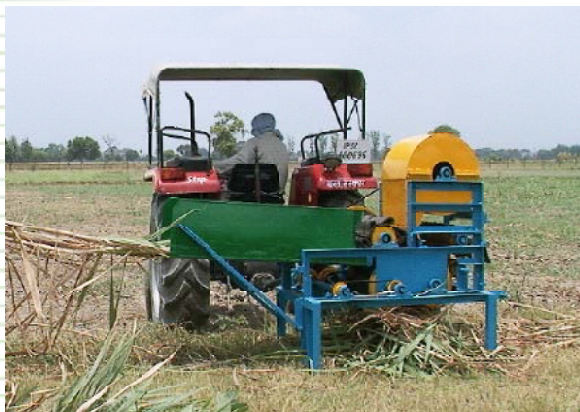
Fig. 7.6: Sugarcane detraser in operation
