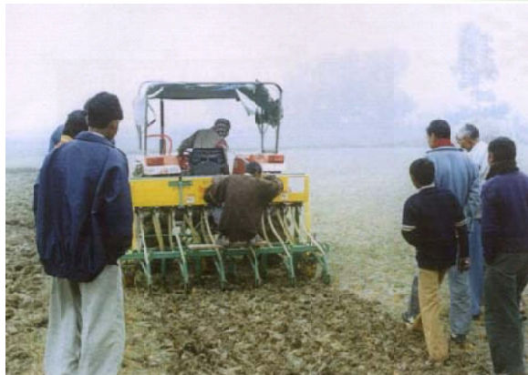
Fig.7.7: Zero Till Drill in operation
