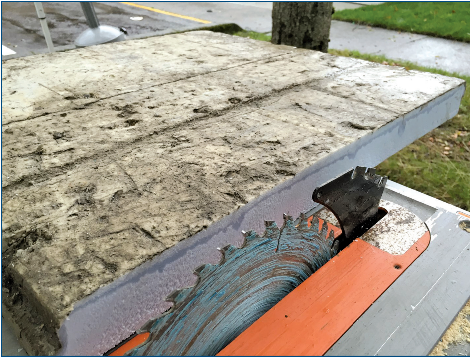
Figure 2 – Thermal conductivity and moisture content measurement sample preparation.
