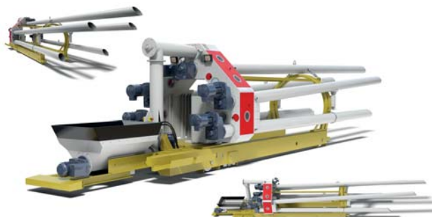
Figure 1: The prototype backfilling machine (CAD modell) with five auger conveyors developed for backfilling the horizontal FE tunnel with granulated bentonite as tightly as possible. The longest auger is 8.5 m long, total length of the device is 11.5 m.
