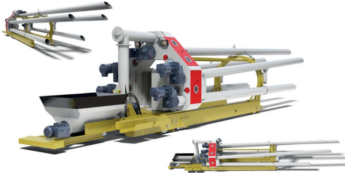
Figure 7. The prototype backfilling machine (CAD model) with five screw conveyors developed for backfilling the horizontal FE tunnel with granulated bentonite as tightly as possible. The longest screw conveyor is 8.5 m long, total length of the device is 11.5 m. (Illustration by McKie, Nagra).
