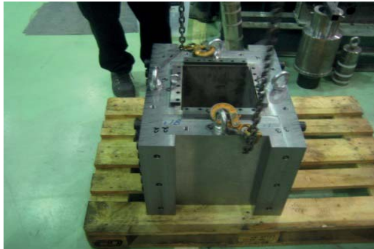
Figure 1. Medium-scale uniaxial backfill block manufacturing mould, for pressing.
