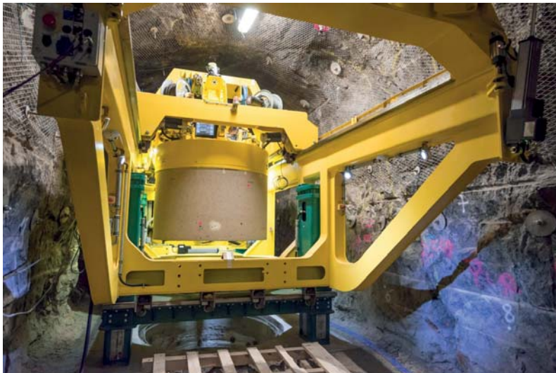
Figure 7. Buffer installation machine operating in ONKALO demonstration tunnel.
