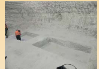
ELSA In-situ compaction tests of specific salt and clay mixtures. © DBETEC and TUBAF
