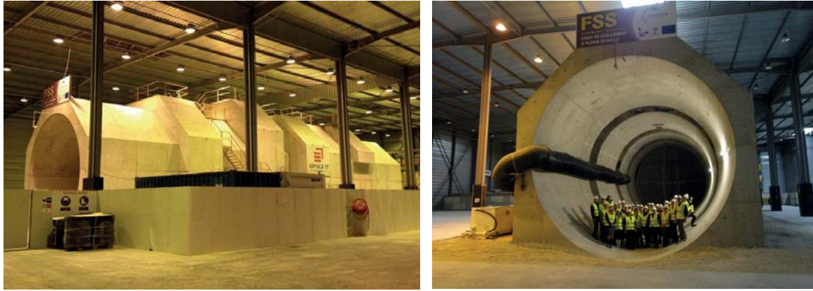
Figure 4 The FSS test box ready for seal construction
