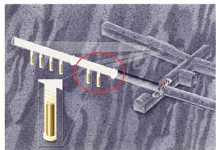
Layout of the Äspö HRL Prototype Repository. Retrieved outer section in red circle above.
