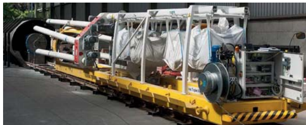
Figure 2: The prototype machine with feeding- and control unit carrying four bigbags. Total length of the backfilling machine including the feeding wagon is 17 m. The photo was taken during a 1:1 scale mock-up test in an off-site workshop. To the left, a dummy-tunnel and a dummy-canister resting on a pedestal can be seen.
