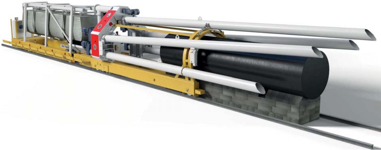
Figure 2. CAD-illustration of the backfilling machine built for the FE Experiment, driving over a dummy canister resting on a pedestal made of bentonite blocks. Total length of the backfilling machine including the feeding device was 17 m. (illustration by McKie, Nagra).
