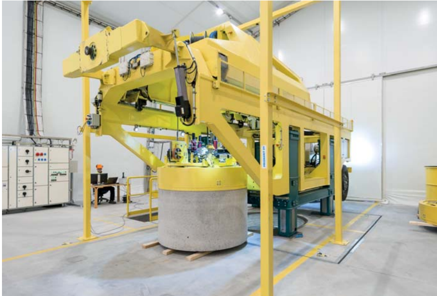
Figure 2. Bentonite buffer installation machine BIM in the ONKALO area test hall.
