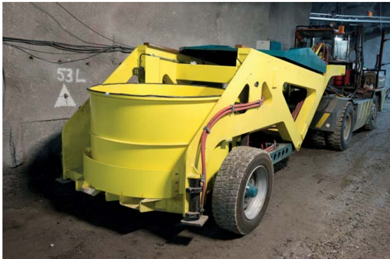
Figure 3. Bentonite transportation device BTB in ONKALO URCF.
