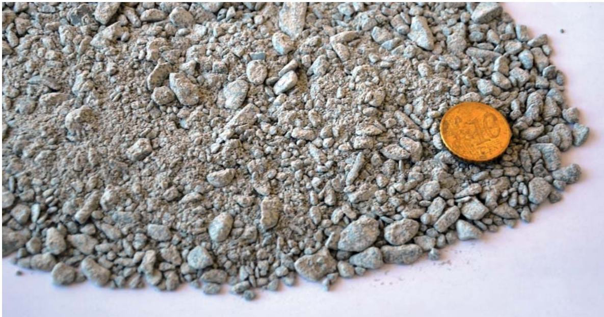
Figure 7. Photo of the granulated bentonite mixture produced.
