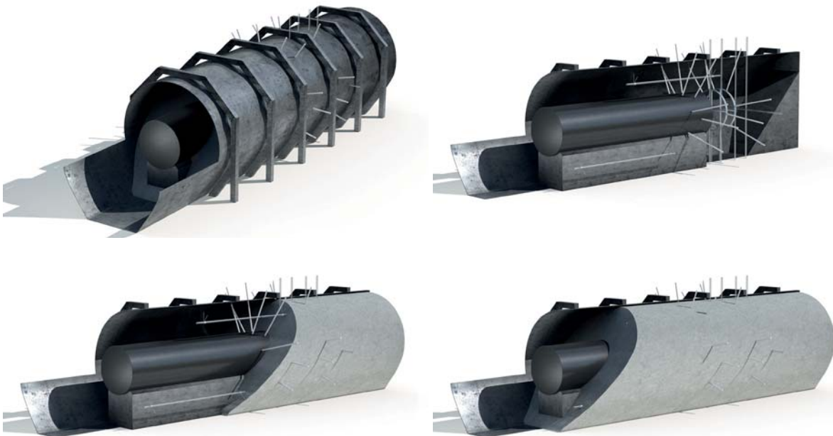
Figure 9. CAD-visualisation of the mock-up test-tunnel showing pipes for density measurements (illustration by McKie, Nagra).
