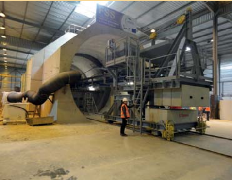
FSS Emplacement of swelling clay core inside the drift model was undertaken in 2014. © Andra
