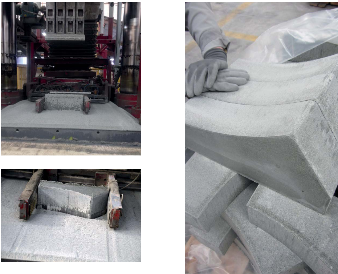
Figure 5: Rectangular and curved blocks after pressing (left) and curved blocks before storage (right)
