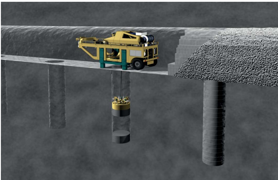
Figure 4. Vertical disposal in crystalline rock (www.lucoex.eu)
