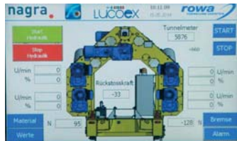
Figure 3: Left photo: Front end of one auger conveyor partially filled with a fuller-type granulated bentonite mixture (GBM). The screw diameter is approx. 25 cm. Right photo: The control panel steers various machine parameters such as the screw turning speed & torque
