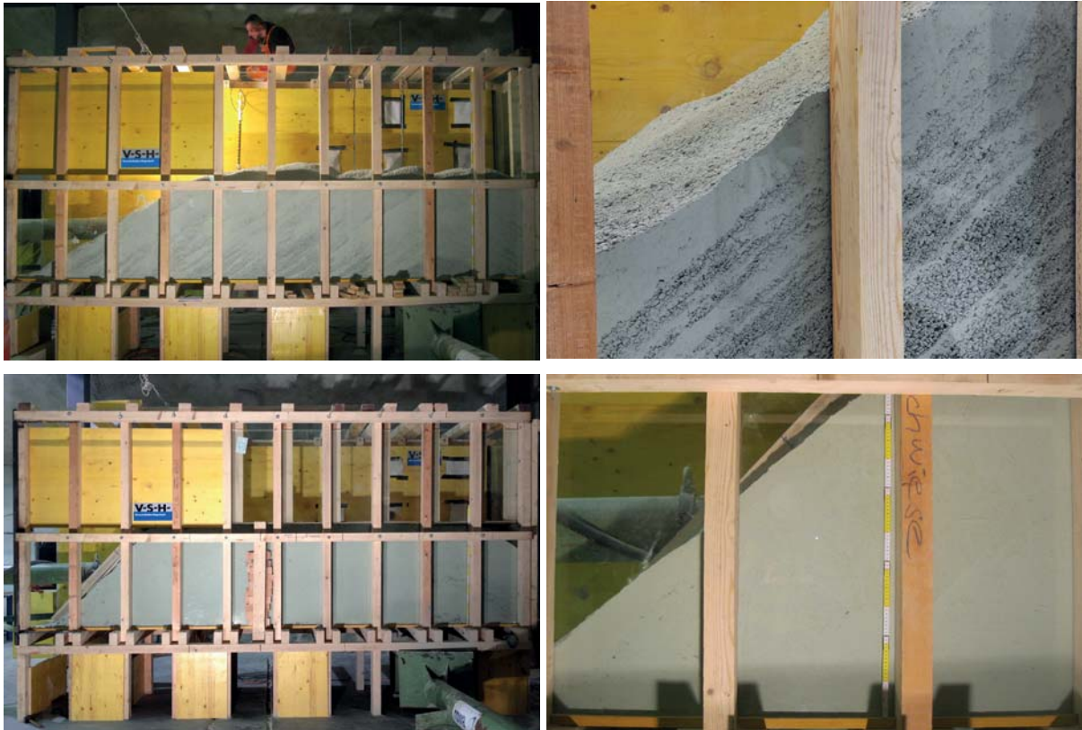
Figure 6. Pre-test B visualised the intensity of segregation effects depending on various measures during backfilling (here: no measures in the top pictures, dry density \rho_d \approx 1.43 \text{ t/m}^3 vs. flexible slope coverage and broader grain size distribution in the lower ones, \rho_d \approx 1.46 \text{ t/m}^3 ).
