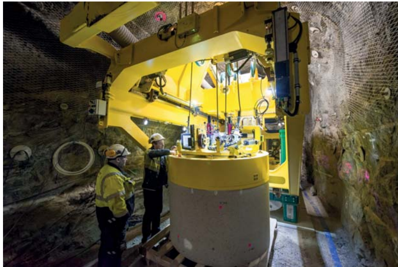
Figure 6. Adjusting of measuring tools of buffer installation machine in the ONKALO URCF demonstration tunnel.
