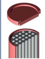
The proposed canister for Lithuanian SNF disposal
