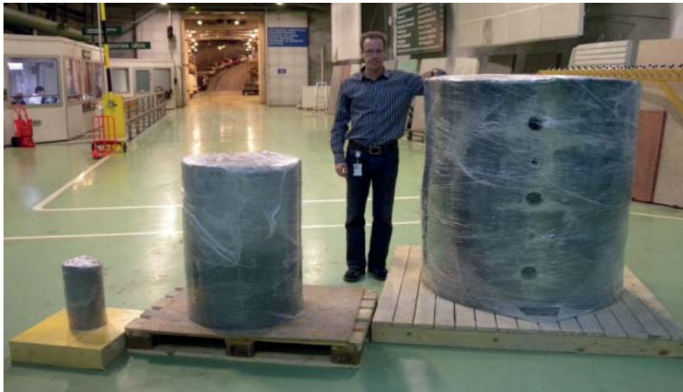
Figure 2. Up-scaling of isostatic compaction of buffer blocks, from small, medium and full-scale.
