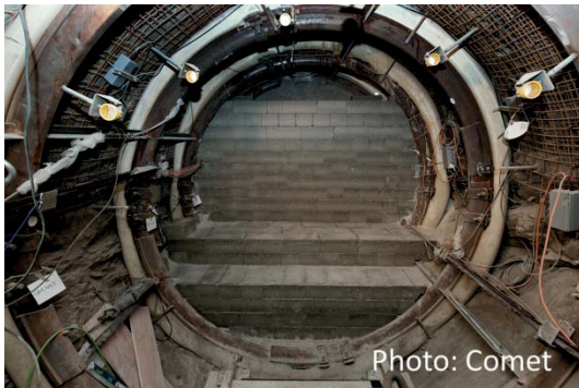
Figure 8: Emplaced bentonite blocks in the FE tunnel: bentonite block wall in the interjacent sealing section and bentonite block pedestal sustaining a heater.
