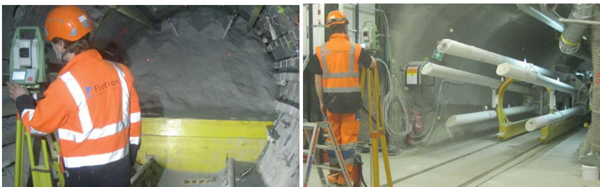
Figure 18. Geodetic survey of slopes (left) and sample-shapes (right) for differential volume and subsequent density calculations (photos: Nagra).
