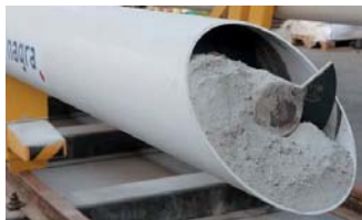
Figure 3: Left photo: Front end of one auger conveyor partially filled with a fuller-type granulated bentonite mixture (GBM). The screw diameter is approx. 25 cm. Right photo: The control panel steers various machine parameters such as the screw turning speed & torque
