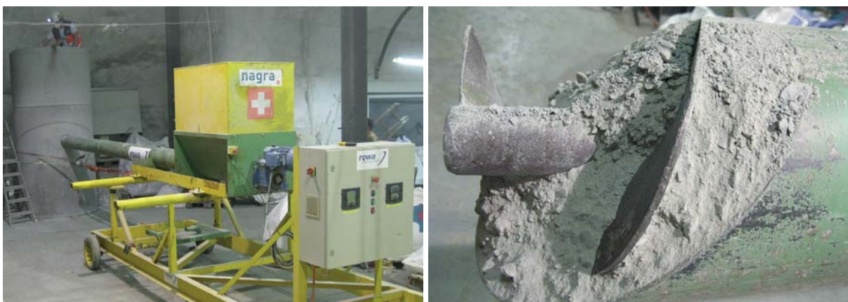
Figure 5. Pre-test A aimed at investigating the potential of pushing the bulk material upwards in a tube of 1.25 m diameter including corresponding parameters.
