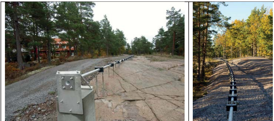
Figure 1. The Äspö deviation facility allows for high precision evaluation of different borehole deviation measurement tools.
