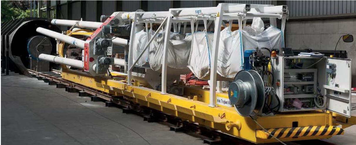
Figure 8. The prototype machine with feeding- and control unit carrying four bigbags. The photo was taken during a 1:1 scale mock-up test in an off-site workshop. To the left, a dummy-tunnel and a dummy-canister resting on a steel pedestal can be seen (photo: Comet).
