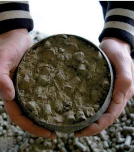
Figure 7. Sample taken from the testing box for dry density determination.
