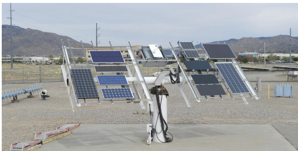
Figure 13: Two-axis solar tracker used for PV module characterization. A variety of different form factors and cell technologies can be characterized simultaneously.
