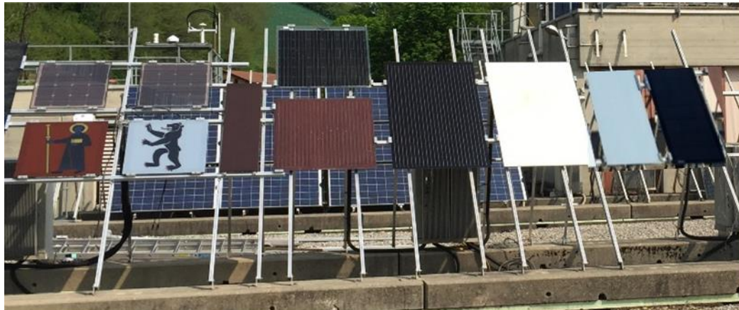
Figure 76: Picture of an outdoor test stand with coloured modules together with some reference modules (Source:[156]). Modules from the left top to the right: textile modules (bifacial), Swiss cantonal flags, deep structured façade module, terracotta module with reference, white module with reference and light grey module with reference.
