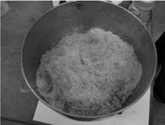
Fig. – 1 Sand mixed with fibers and medium containing bacteria
