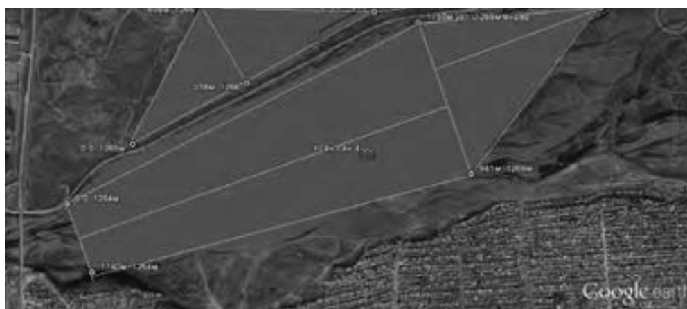
Figure 8. Flow control water reservoir-I /Google Earth/ Water reservoir for flow control Tuul river between 2 bridges Yarmag and Songolon will be with length 2470m, perimeter 5571m.
