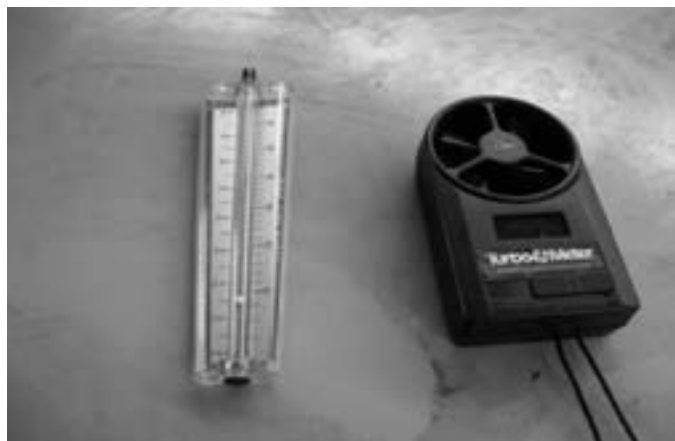
Fig. – 4 Digital Turbometer wind speed indicator and Dwyer wind meter
