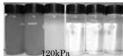
Figure 8. Pictures of sample cells (Right is higher water pressure)
