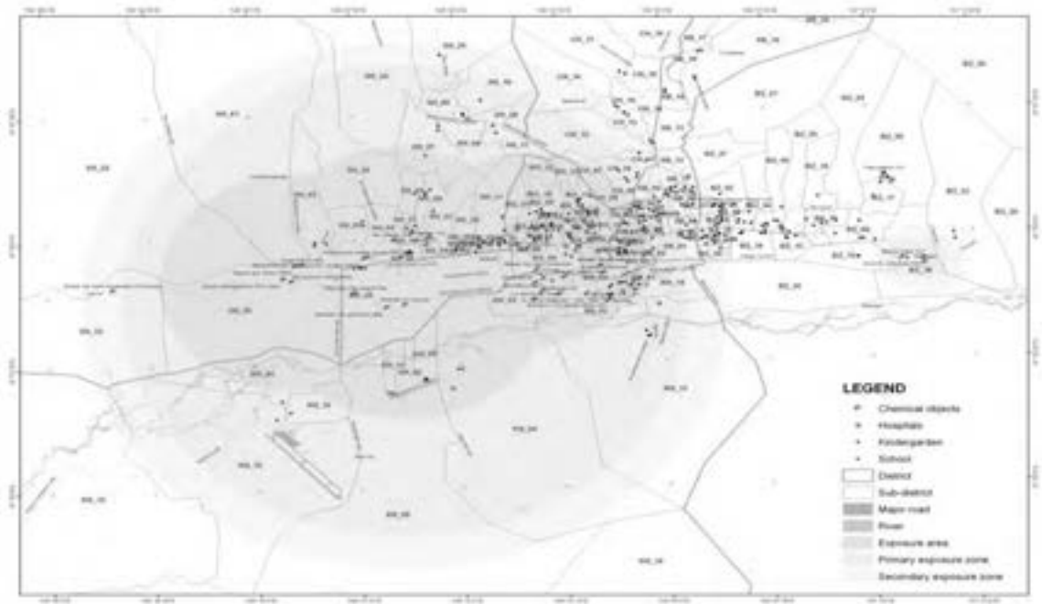
Figure 2: Exposure and hazard area by the direct release of toxic and dangerous liquids and volatile substances from dangerous chemical objects in Ulaanbaatar
