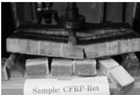
(c) Failure pattern of CFRP-retrofitted masonry wallet
