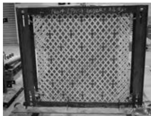
(b): PP-band retrofitted wall in the laboratory.
