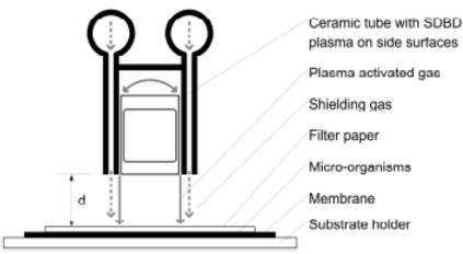
Figure 1: Electrode system and substrate composition
