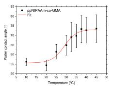
Figure 1: Water contact angle measurements of pp-NiPAAm-co-GMA in dependence on the different temperatures.
