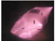
Figure 1: Generated plasma inside the packaging bag
