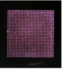
Figure 1 : Array of 1024 MHCDs of 100 µm diameter operating in Helium at 350 Torr
