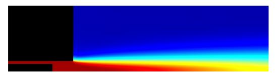
Figure 1: Image of the argon concentration flowing from the end of the plasma jet applicator
