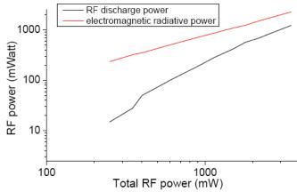
**Fig 1:** *RF power deposited in the helium plasma jet compared to radiated RF power.* In term of applications, this work demonstrates that plasma jets generated by radiofrequency excitation are always accompanied by RF radiation. This last point is not necessarily a negative because some treatments use radiofrequency to treat tumors [1].
