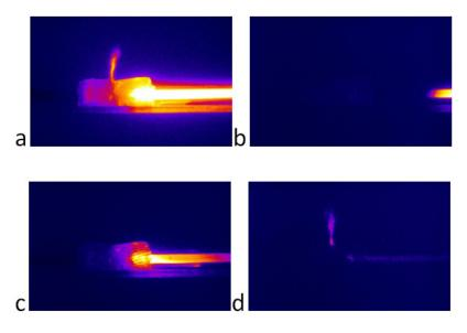
**Figure 1:** Plasma bullet propagation in agarose gel with an L-type tube: images taken with a high-speed ICCD camera a) exposure time 20 us b-d) exposure time 100 ns, delays b) 0.3 us, c) 0.6 us, and d) 1.5 us.
