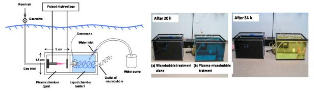
Figure 1 Experimental setup of P-MS.
