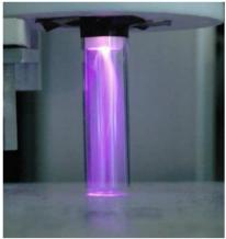
Figure 1: PlasmaStream helium atmospheric pressure plasma jet system
