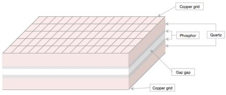
Figure 1: The DBD lamp prototype design principle (80 mm × 120 mm × 6 mm)
