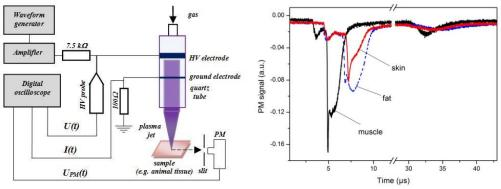
Figure 1: Experimental set-up used for temporal dynamics studies and typical PM traces.
