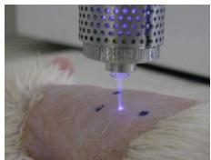
**Figure 1:** A device photograph in action. The skin of living rat was exposed to plasma for 15 minutes without any signs of tissue damage or inflammation.
