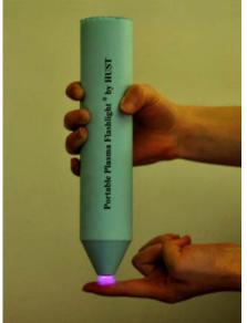
Fig. 1. Photograph of the air plasma flashlight
