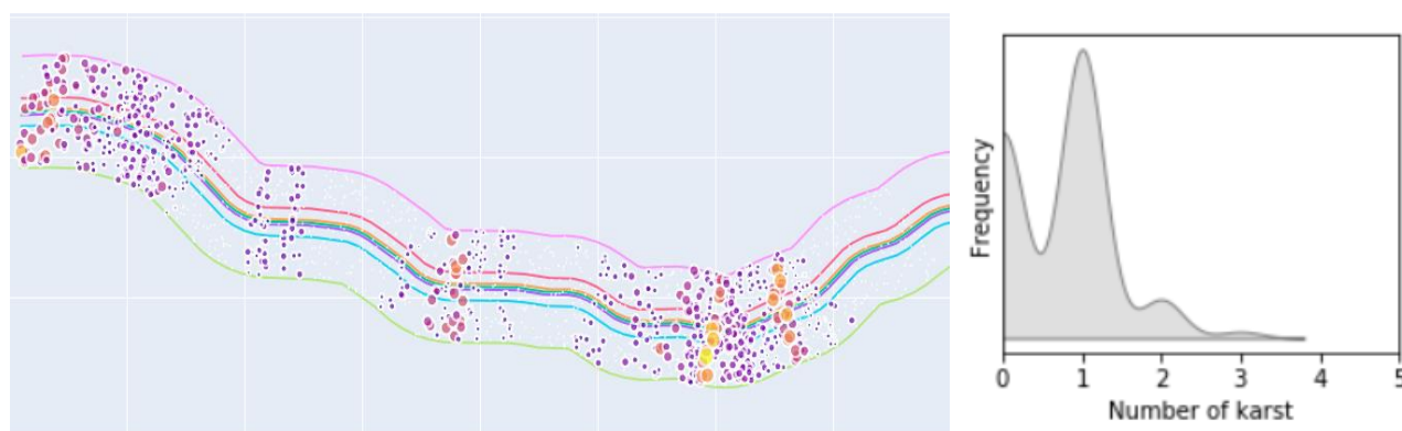
Figure 1. left image shows the karst position derived from the stochastic analysis plotted on the motorway project the right figure shows the kernel density distribution of karsts intercepting the project site for a particular sector
