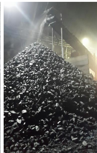
Figure 2: Pre-crushing and screening (0/150 mm) in tunnel
