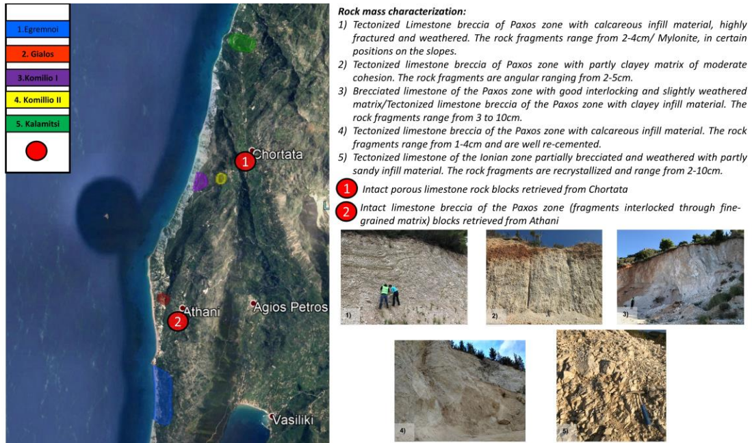
Figure 1: Rock mass characterization of the sites visited in western Lefkada
