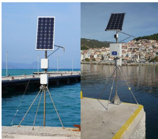
Figure 1: Two out of the three tide gauge stations that have been installed in Kos (left) and Plomari, Lesvos (right).
