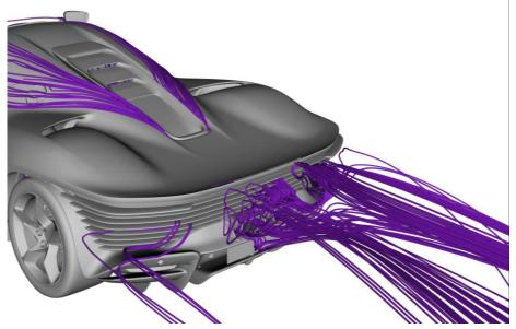
Fig. 14 - Interaction between the apertures on the sides of the backbone and the rear grille to guarantee the required cooling flow to the engine compartment
