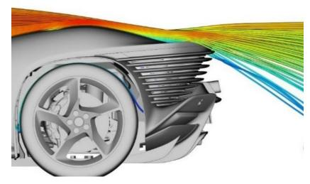
Fig. 20 - Pressure distribution on the rear bodywork and the flow to the spoiler
