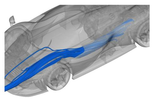
Fig. 13 - Side radiator intakes integrated into the doors
