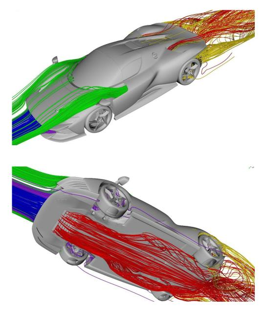
Fig. 12 – Car cooling flows and heat evacuation: blue/red engine and air con water, green/yellow enginegearbox-clutch, purple brakes
