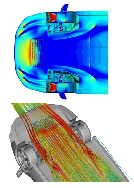
Fig. 19 - Aerodynamic sealing effect of the vortex generator on the front underbody
