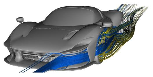
Fig. 16 - Synergy between vented side bumper and wheel to manage the flow along the flanks: the flow continues to hug the car's flanks, reducing the size of the car's wake
