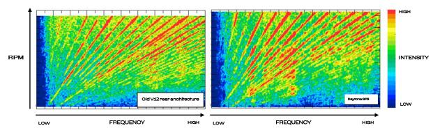
Fig. 9 - The sound pressure spectrum in the cabin as revs rise. The unusal intake layout lends the classic harmonics of the Ferrari V12 a greater intensity in mid frequencies, yielding a signature timbre that only adds to the car's sporty allure
