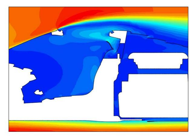
Fig. 24 - Interaction between the windshield nolder and the cabin: the turbulent wake is deflected upward to prevent it re-entering the rear area of the cabin
