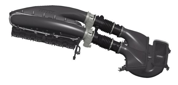
Fig. 4 - Intake assembly
