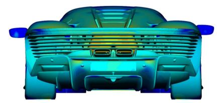
Fig. 23 - Double central diffuser: the central bridge is flanked by a more external diffuser volume that enhances its efficiency
