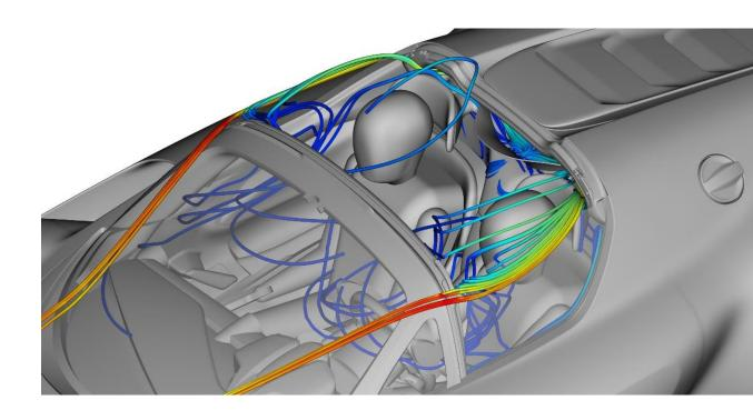
Fig. 25 - Turbulent flow captured by the central windstop and vented through slots in the upper trim
