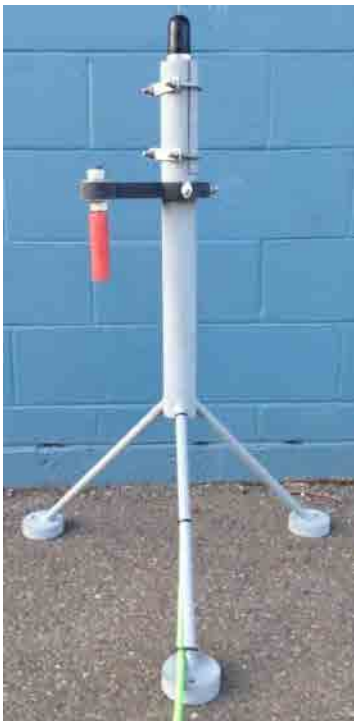
Figure 6: A Hydrophone tripod mount that supports the hydrophone at a height of one metre above the seafloor.
