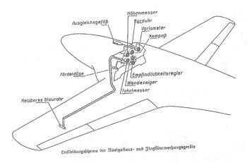
Drawing from LDv.557 Teil 3 showing the Pitot tube and gages and the Turn & Bank nozzle and gage
