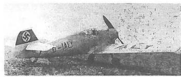
Here we see the V-4 and just forward of the windscreen the Turn & Bank nozzle is discernible as a light line due to Sun hitting it but the shadow of it is also seen as two lines. This seems to have been the last to mount the sensor here.
