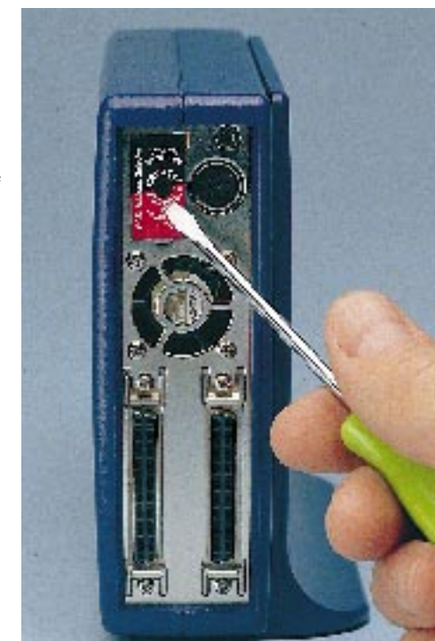
Every SCSI device must be assigned a unique SCSI ID, from 0 to 7
