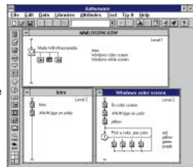
With Authorware, creating applications is carried out using a flowchart method
