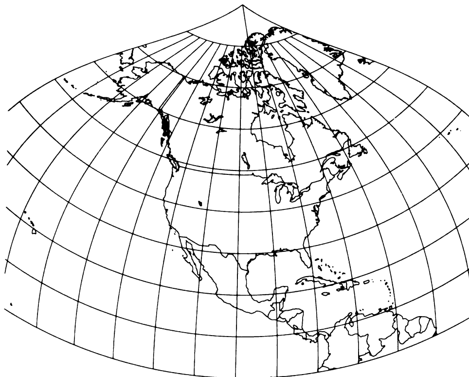
FIGURE 27.—Bonne projection with central parallel at lat. 40° N. Called a pseudoconic projection, this is equal-area and has no distortion along central meridian or central parallel. Popular in atlases for maps of continents until mid-20th century.
