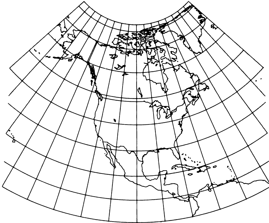
FIGURE 20.—Albers Equal-Area Conic projection, with standard parallels 20° and 60° N. This illustration includes all of North America to show the change in spacing of the parallels. When used for maps of the 48 conterminous States standard parallels are 29.5° and 45.5° N.
