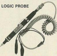
Compatible with all logic families using a 4 to 15V power supply. Thresholds automatically programmed. Visual indication of logic levels to show high, low, bad level or open circuit logic pulses.
