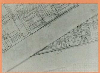
FIG. 2—DRAW YOUR PATTERN on a sheet of tracing paper that has been attached to a sheet of graph paper. The graph paper should have 0.1-inch spacing. For double-sided boards use a second sheet of tracing paper.
