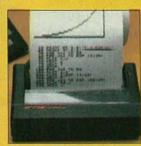
ZX PRINTER: The Sinclair ZX Printer will work with your ZX81, or ZX80 with 8K BASIC. It will be available in the near future and will cost less than \$100.
