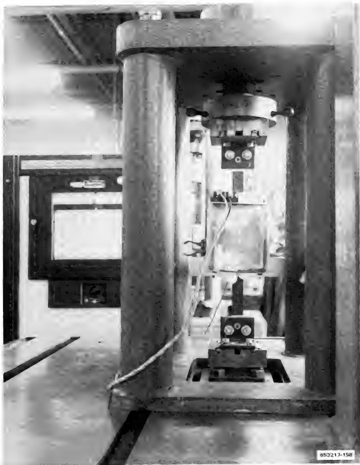
Figure 11-4 Furnace Arrangement for R = 0.1 Fatigue Test at Elevated Temperature
