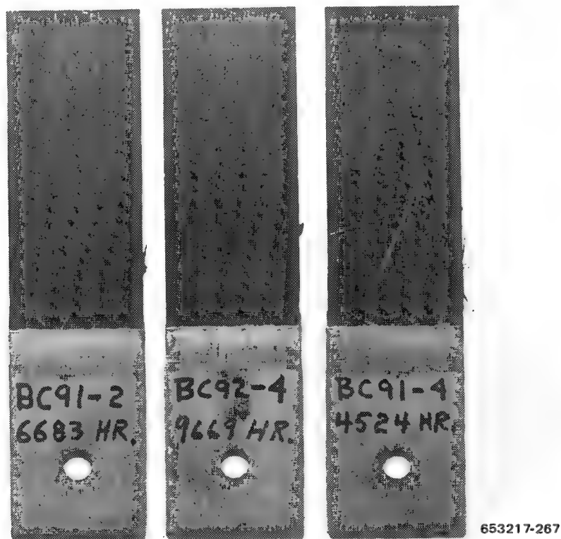
Figure 12-67 G/E Long-Term Specimens that were Removed from Test Before Completion of 10,000 hr of Exposure. (Increasing levels of damage in the specimens are visible in moving from left to right)
