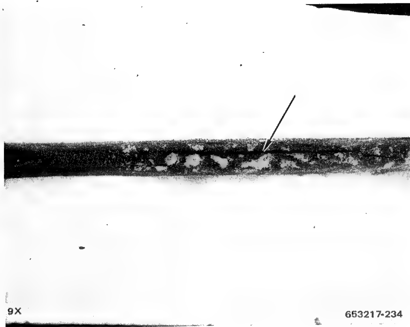
Figure 12-34 Edge Cracking (arrow) in Specimen DF81-5, G/PI, Notched, After 100-hr Simulation Exposure at 505 K (450° F)
