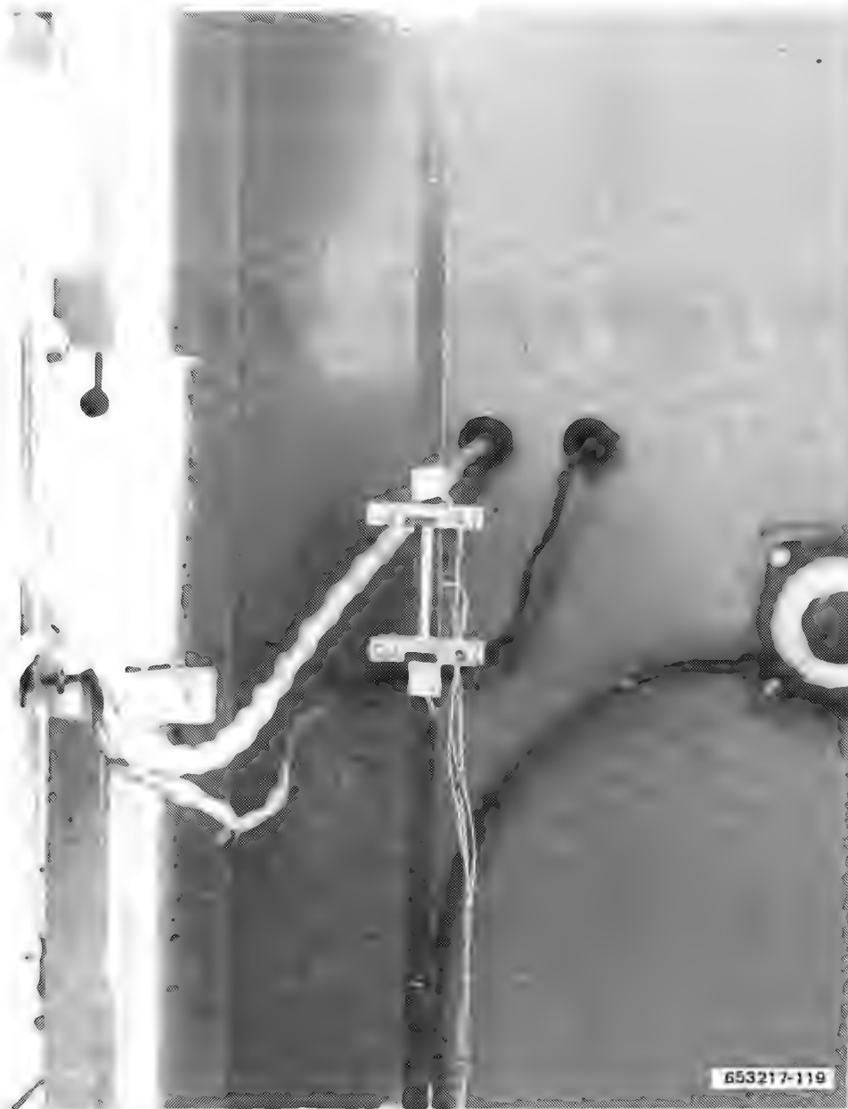
Figure 10-4 Creep Specimen with Platinum Sliding-Strip Extensometer and Thermocouples Attached
