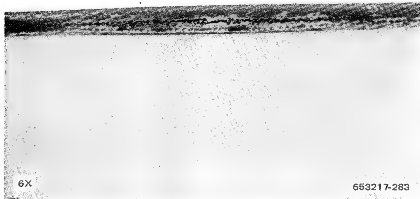
Figure 12-83 B/Al Long-Term Specimen EC91-1 After 10,000 hr of Flight Simulation Exposure Showing Edge Cracking in Heated Zone
