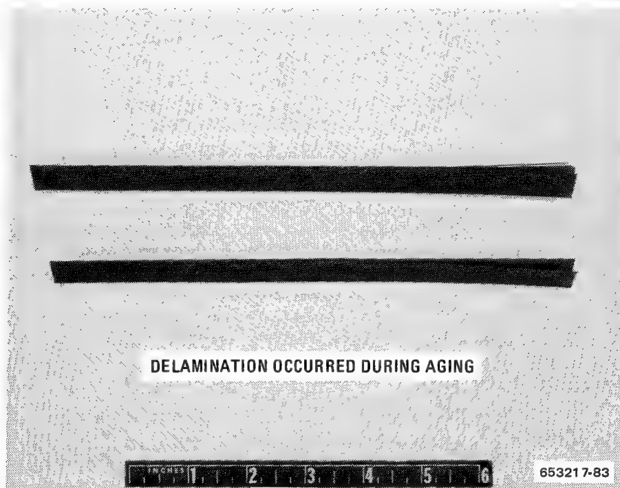
Figure 8-12 Crossplied B/E After 10,000 hr of Thermal Aging at 450 K (350° F) in 1 atm Air
