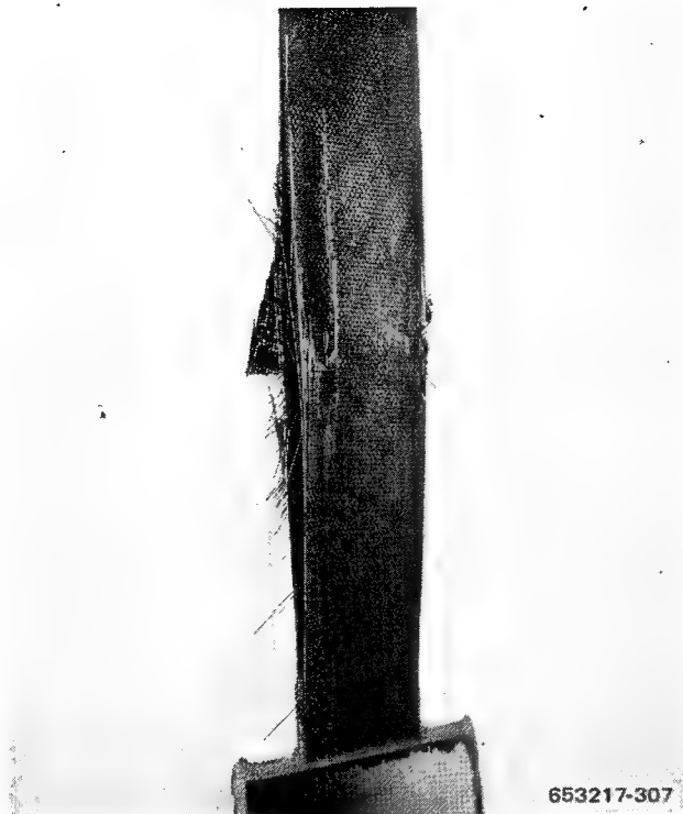
Figure A-1 Heated Area of B/PI Short-Term Specimen After Only 7 hr of Flight Simulation Exposure at 505 K (450° F)
