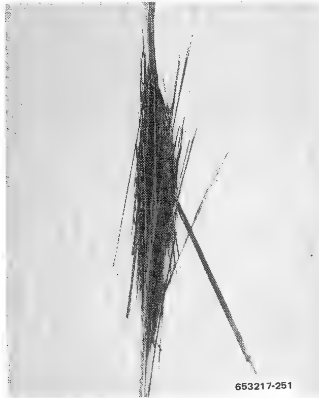
Figure 12-51 Edge View of G/E Long-Term Specimen BC91-4 Showing Exposed and Broken Graphite Filaments and Extensive Delamination. (Specimen was removed from test after 4524-hr)
