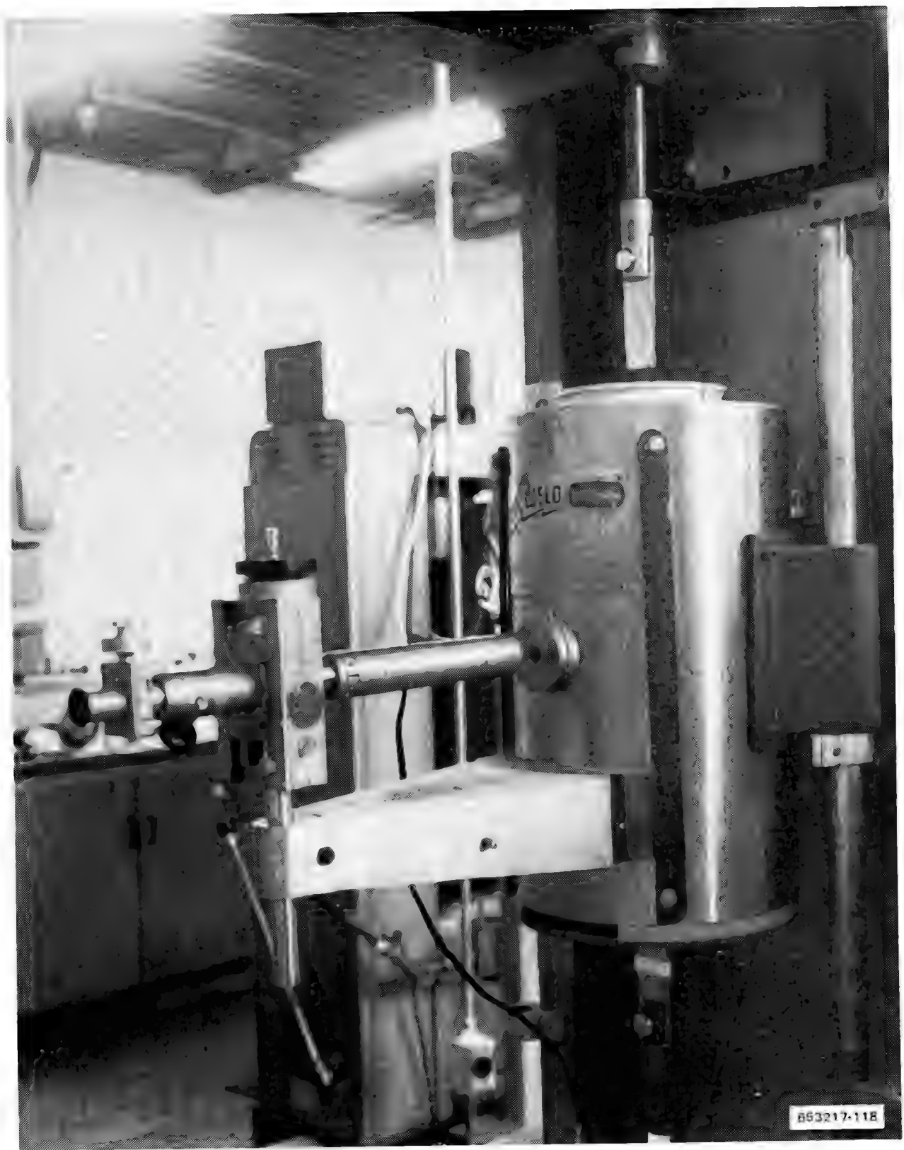
Figure 10-3 Furnace Mounted Filar Micrometer Microscope for Creep Measurements
