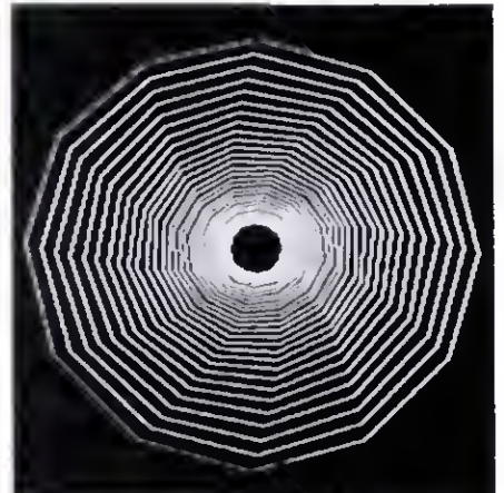
Photo 4. When you specify a number of sides in Polygon/BAS greater than 20, it produces a nested, rotating spiral. Here, SD = 12.
