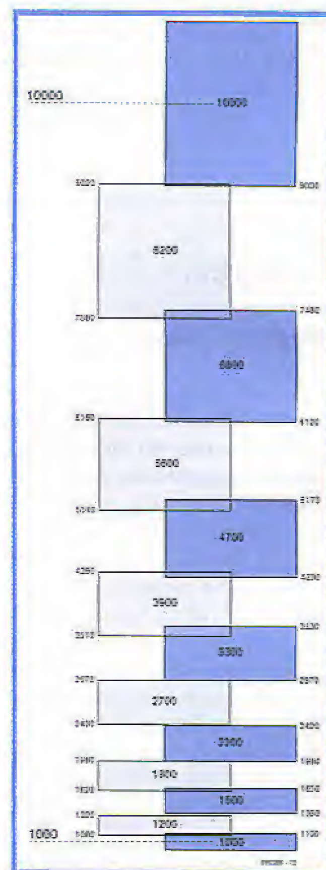
Figure 2. Tolerance regions for the E12 series. Because the values are rounded, the regions do not join exactly but overlap a little or leave a small gap.
