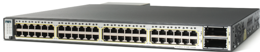
Figure 1. Cisco Catalyst 3750E-48TD Switch
