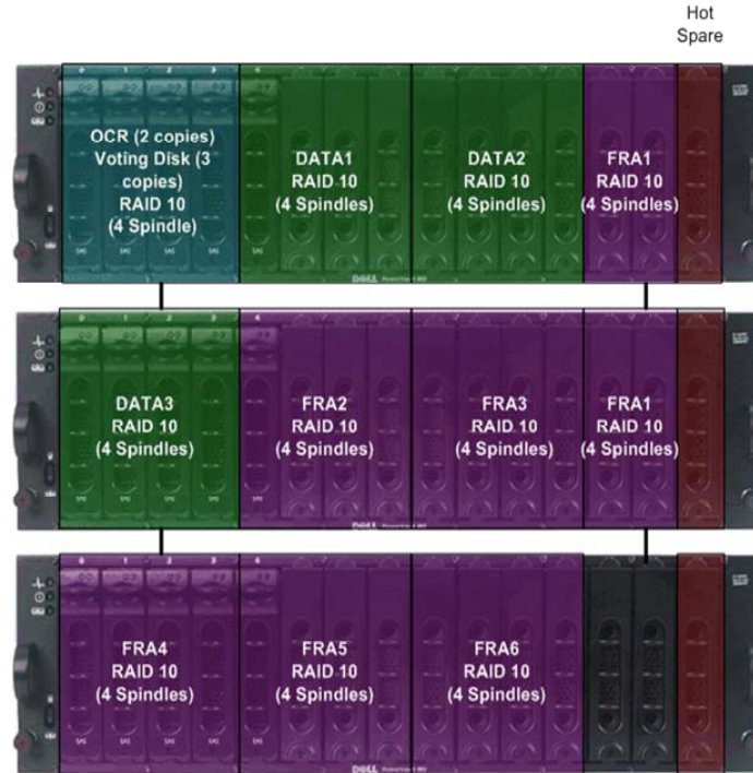
Figure 6 - Separation of Disk Groups and Virtual Disks within a PowerVault MD3000i Storage Array and two MD1000 Expansion Units
