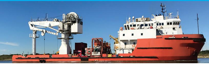
**THE SUBSEA RESPONDER I** is a DP2 Saturation Diving Support Vessel, also capable of inspection, maintenance and repair (IMR) work.
