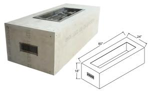
Size: 60" X 24", 18" tall Insert: 30" X 12" H-Burner Hardie Board Cladding SQ FT: Side: 22.5 - Top: 8.1 - Total: 30.6 Includes 10% Buffer
