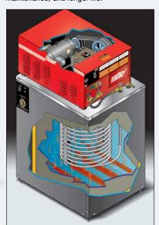
Water is heated in a **Stainless Steel Coil** submerged in a tank of water solution for efficient heat transfer and instant hot water with the pull of the trigger; a **layer of oil** rests on the surface of the tank water solution for additional retention of heat and to prevent evaporation.
