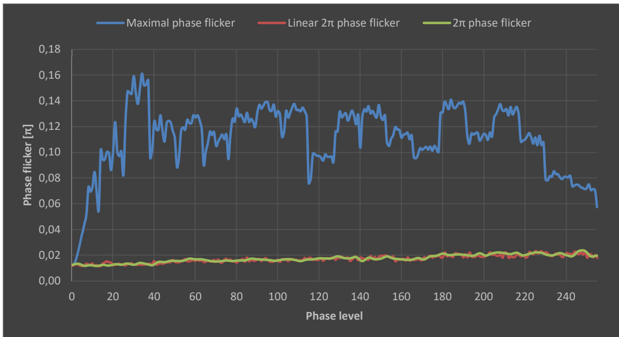
Figure 5. Phase flicker (peak to peak) calibration measurements for @1064 nm with PLUTO 2.1 NIRO 023
