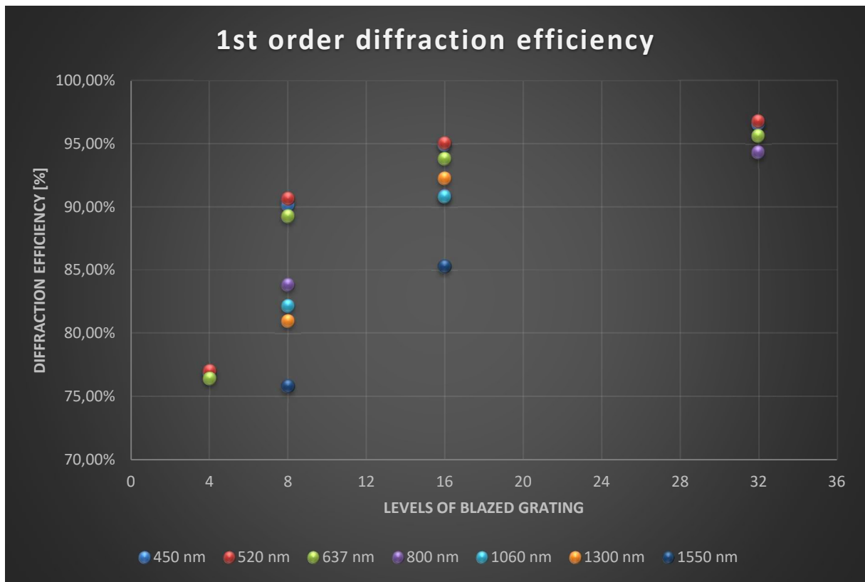
Figure 11: Measured diffraction efficiencies of the 1st order of blazed gratings with different spatial frequencies for defined wavelengths.
