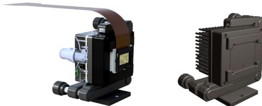
Figure 13: Display mounts compatible with Thermal Management Systems
