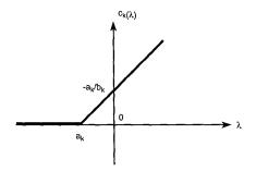
Fig. 8. Capacity function on arc  $(s, s_k)$ .
