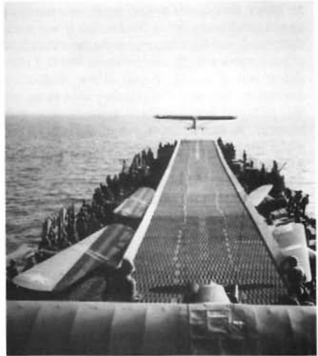
Liaison aircraft taking off from makeshift runway on an LST during Anzio landing (January 1944).
