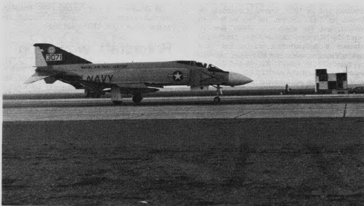
Lt. Jim Ellis making a touch-and-go landing in Navy F-4 at Crows Landing with MLS Elevation in background.
