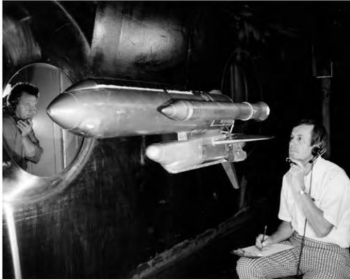
An engineer checks a scale model of the transportation system before testing in NASA Glenn's 10 by 10-foot wind tunnel in 1975.
