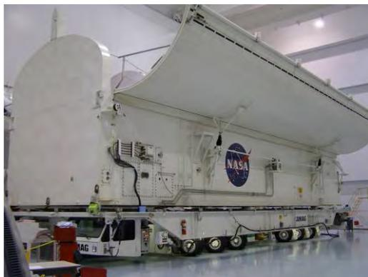
Payload Canister on Canister Transporter in the Space Shuttle Processing Facility.
