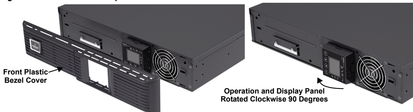
Figure 8 Remove the front plastic bezel cover
