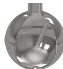
Fig 3. Cross-section of spherical test cell, showing thermowell
