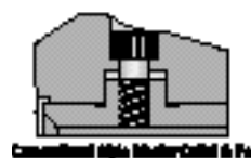
Conventional Style Master Collet & Pad
