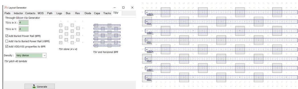
Figure 15: TSV generator and BPR aligned to the TSV grid in Microwind, and associated nTSV array in very dense mode (tsv-4x4-very-dense.MSK).
