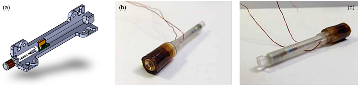
FIG. 16. A schematic of the thruster head mounted in a CubeSat Rail (a), and pictures of a thruster head [(b) and (c)]. In a vacuum arc, the discharge is initiated on the cathode surface. Plasma is generated depending on the material and surface structure in so-called arc spots. These micro-plasmas expand into the vacuum and allow current to flow directly from the cathode to the anode along a lower resistance plasma discharge path.
