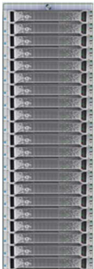
Figure 1. Rack loading with twenty ProLiant DL380 Gen9 servers using 800W Flex Slot power supplies @ 208 VAC.
