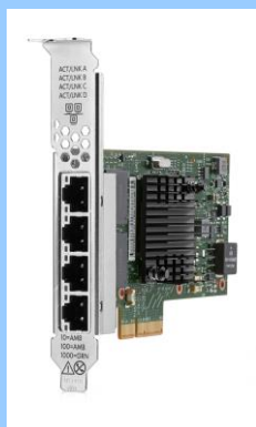
HPE Ethernet 1Gb 4-port BASE-T I350-T4V2 Adapter
