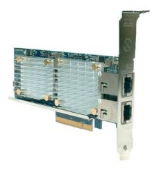
The Broadcom NetXtreme 10GBaseT Network Adapter Family for System x® features a robust, standards-based portfolio that delivers economical Ethernet features in an industry-standard PCIe Gen 2 form factor, and exclusive ML2 form factor.
