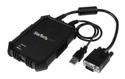
This rugged and portable USB crash cart adapter lets you turn your laptop into a portable console for accessing servers, desktops and laptops, as well as ATMs, kiosks or any computing device that features both VGA and USB ports.
